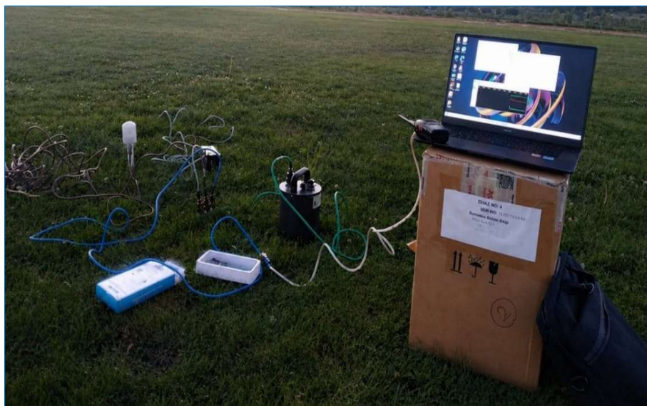
Fig. 4. Microtremor measurement system (GURALP broadband CMG-6TD)
