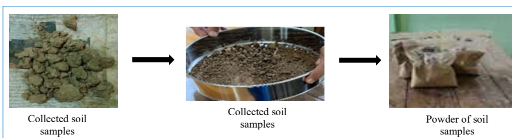
Fig 2. The preparation of soil sample
