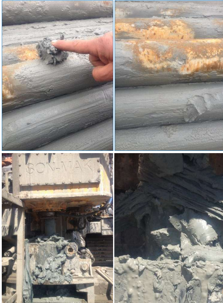
Fig. 5. Views of clays sticking on drill rods and decomposed clays
