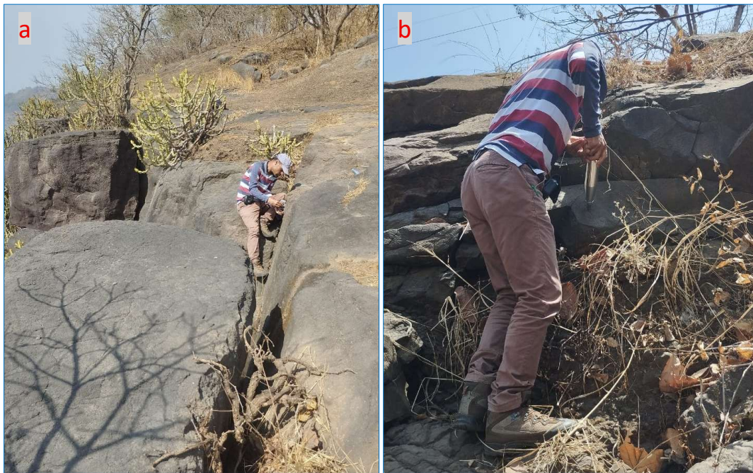
Fig. 3. Assessing geomechanical parameters of in situ rock mass: (a) measuring orientations of discontinuities (joints) of rock and slope geometry using Brunton Compass and (b) achieving rebound nos. of each joint using Schmidt hammer for strength of rock mass
