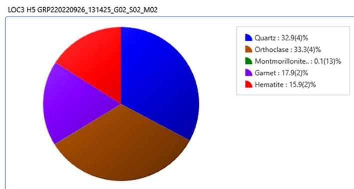
Fig. 12. XRD quantitative analysis pie chart weight % of minerals in sample 5
