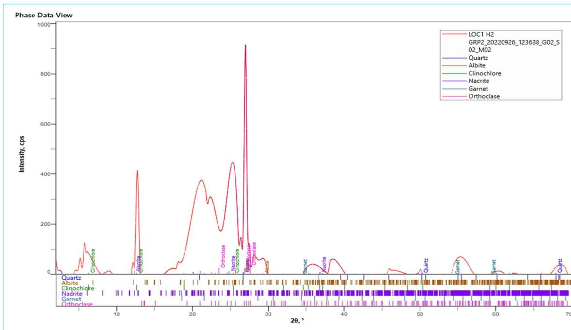
Fig. 5. XRD qualitative analysis peak plot of intensity (cps) against 2θ° sample 2
