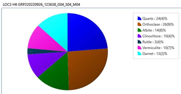
Fig. 14. XRD quantitative analysis pie chart weight % of minerals in sample 6
