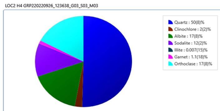
Fig. 10. XRD quantitative analysis pie chart weight % of minerals in sample 4
