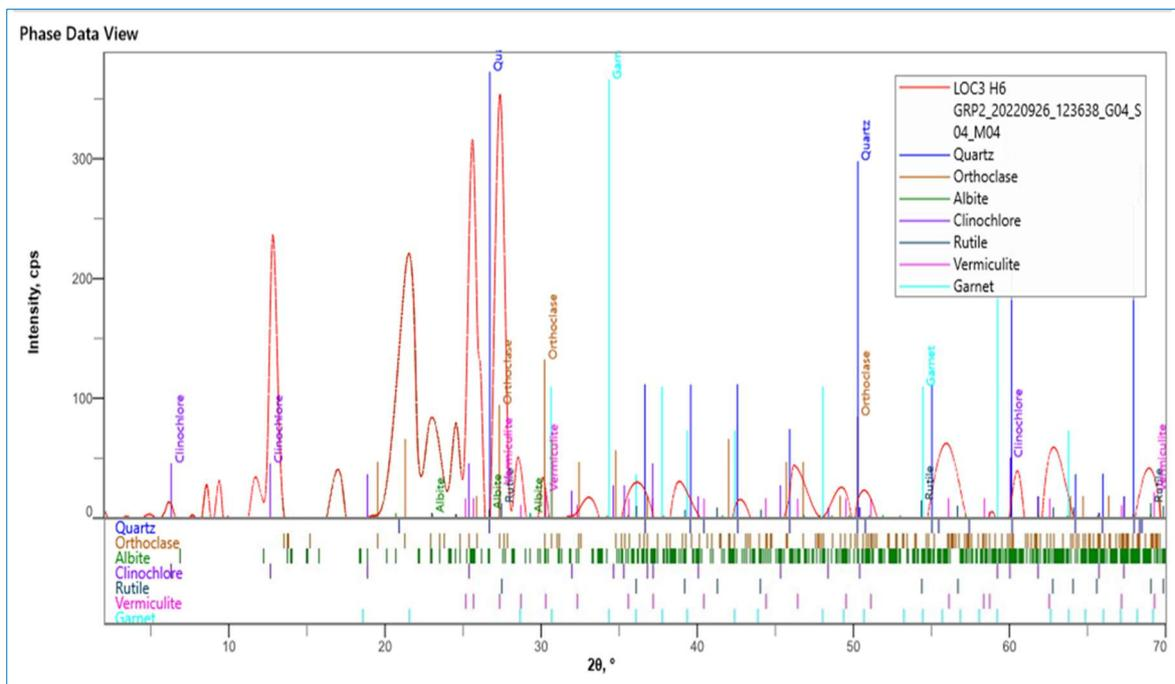
Fig. 13. XRD qualitative analysis peak plot of intensity (cps) against 2θ° sample 6
