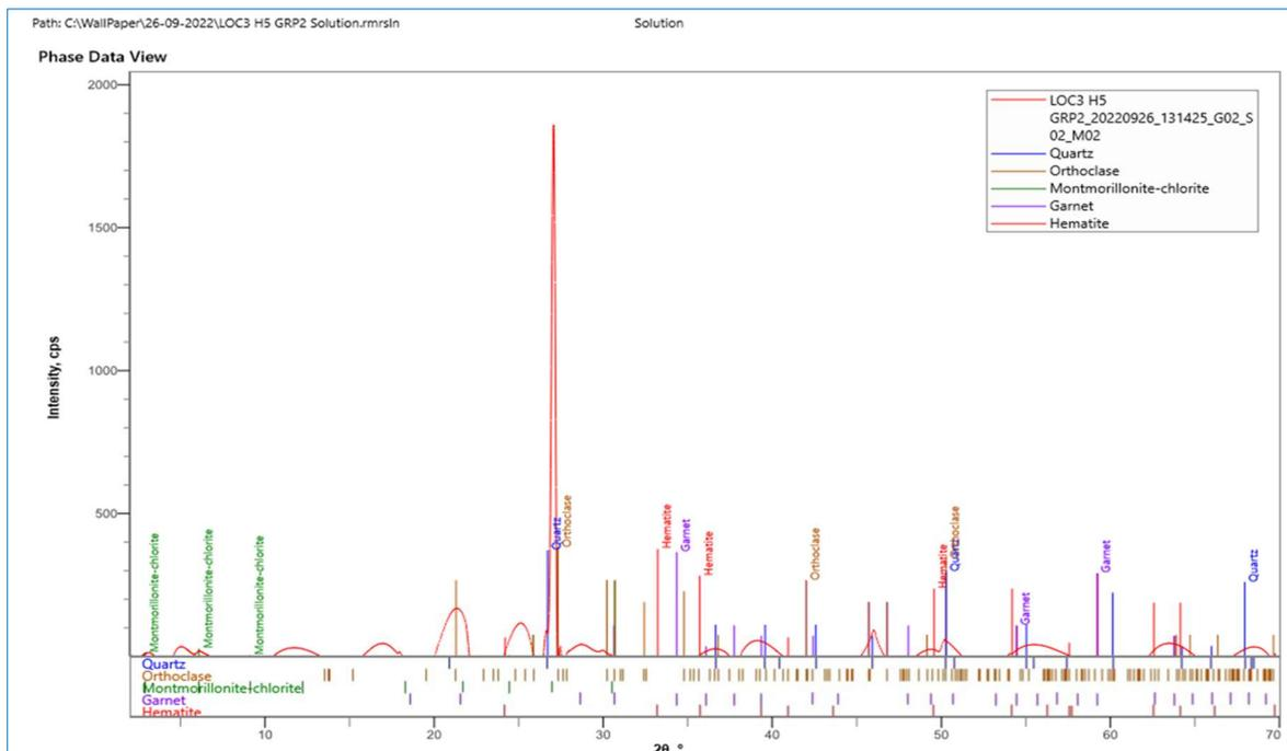
Fig. 11. XRD qualitative analysis peak plot of intensity (cps) against 2θ° sample 5
