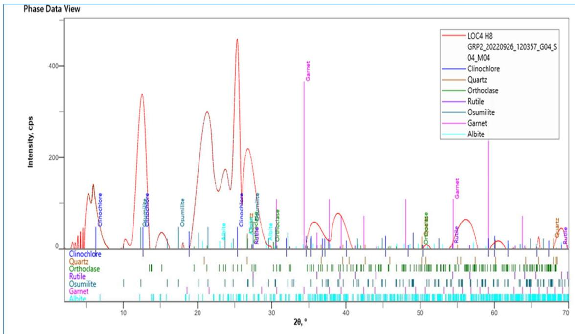
Fig. 17. XRD qualitative analysis peak plot of intensity (cps) against 2θ° sample 8
