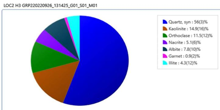
Fig. 8. XRD quantitative analysis pie chart weight % of minerals in sample 3
