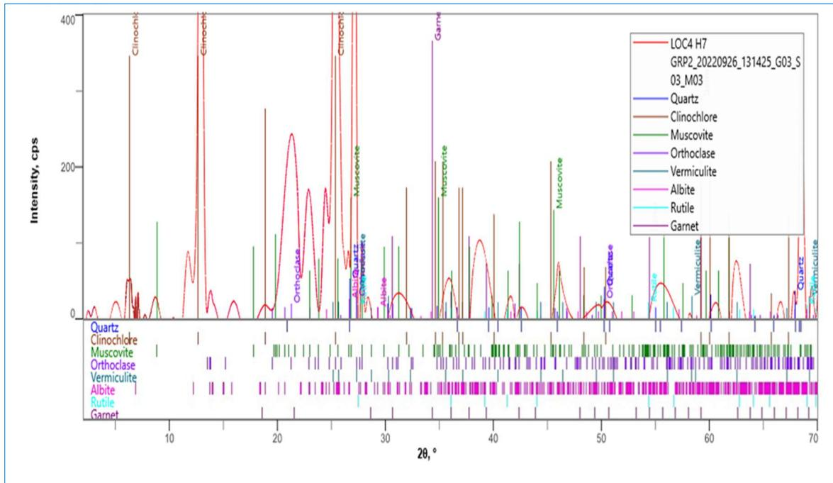
Fig. 15. XRD qualitative analysis peak plot of intensity (cps) against 2θ° sample 7
