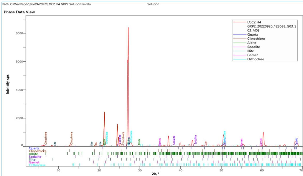
Fig. 9. XRD qualitative analysis peak plot of intensity (cps) against 2θ° sample 4
