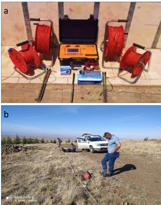
Fig. 3. A view of the device used in geophysical resistivity study (a) and the field measurements (b)
