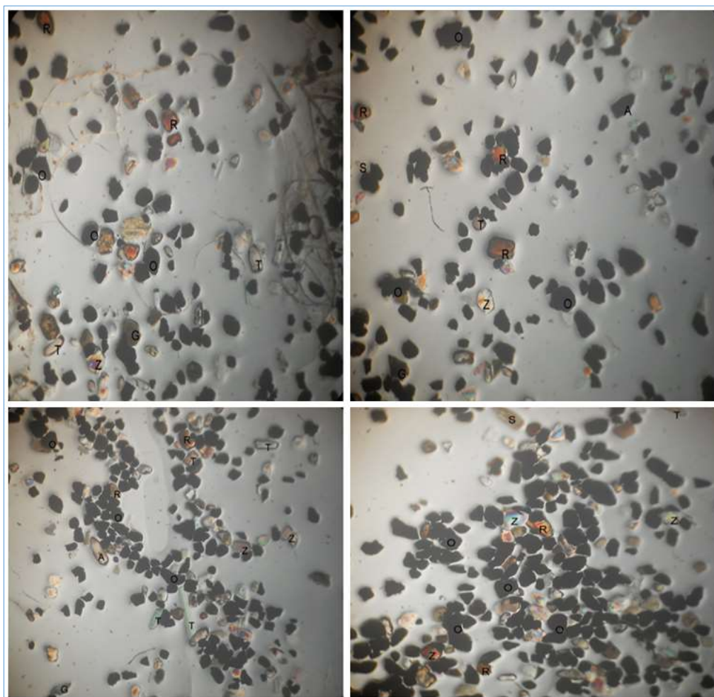
Fig. 8. Photomicrograph of Heavy Mineral analysis of Sandstone located at Ajegunle, Papalanto and Ifon outcrops (30x). Legend: Z is for Zircon, R is for Rutile, T is for Tourmaline, G is for Garnet, S is for Staurolite, and O is for Opaque. The ZRT index is calculated by adding Z, R, and T, and then dividing this sum by the total opaqueness. The result is then multiplied by 100
